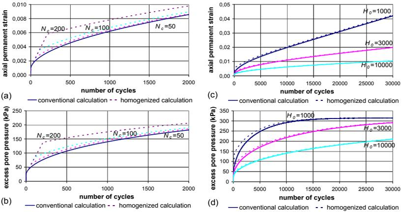
**FIG. 2. Comparison of conventional and homogenized calculations: (a) permanent strain / (b) excess pore pressure for  $H_0 = 1000$  and  $N_c = 50, 100, 200$ ; (c) permanent strain / (d) excess pore pressure for  $H_0 = 1000, 3000, 10000$  and  $N_c = 200$ .**
