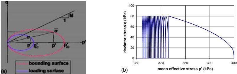
**FIG. 1. (a) Representation of bounding and loading surfaces in  $(p', q)$  plan. (b) Simulation of an undrained triaxial test on a normally consolidated clay under one-way cyclic loading in  $(p', q)$  plan.**
