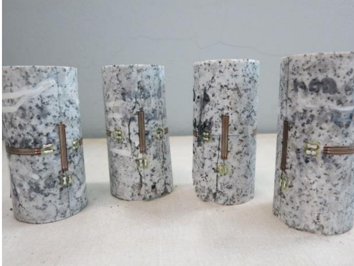
Fig.2 – Sidobre granite. Compressive test on cylindrical specimens, D=50 mm, H=100 mm
