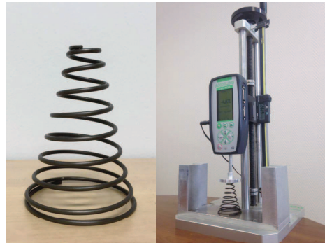
Fig. 12. Conical spring manufactured and measuring equipment
