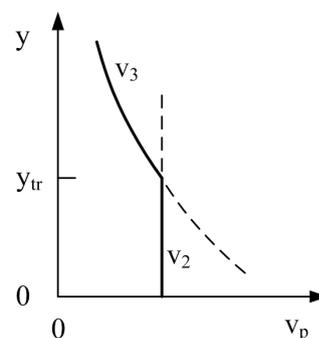
**Figure 2** | Turbulent plumes, flat ( $v_2$ ) vs round ( $v_3$ ). The competition for more effective mixing (the smallest  $v$ ) dictates the transition from flat plume to round plume (and not from round to flat).
