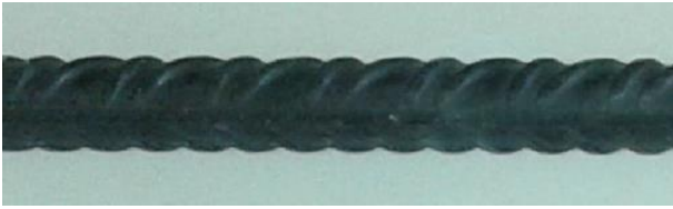
Figure 7. HA12 steel bar.
