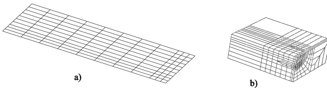
**Fig. 2** Meshes for semi-elliptical surface crack in a rectangular membrane: a) one-quarter of the global (shell) model mesh without a crack, b) one-quarter of the submodel mesh with a semi-elliptical crack.
