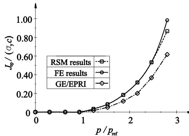
**Fig. 22** Comparison of FE and GE/EPRI  $J$  results with the proposed reference stress-based  $J$  estimations ( $R_m/t = 4.8$ ,  $c/a = 2.08$ ,  $a/t = 0.8$ )
