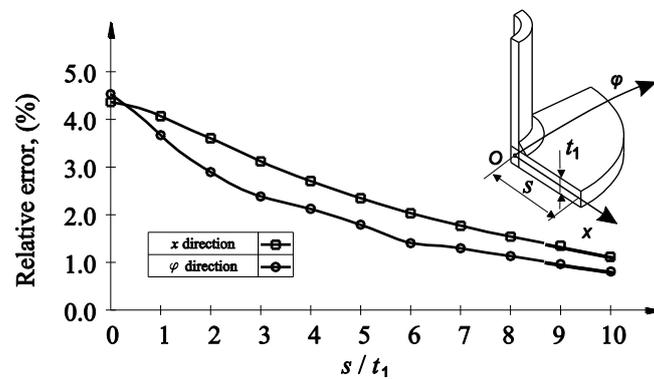
**Fig. 18** Variations of the difference in radial displacements distribution of mid surface along a longitudinal and circumferential cross-section of the pressure vessel obtained from the shell model and the full 3D solid FEA
