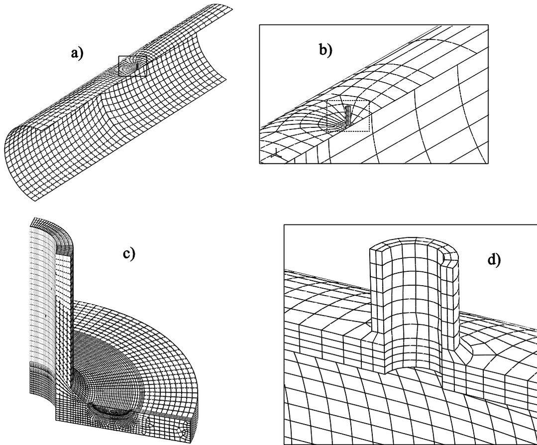
**Fig. 17** Typical FE meshes for a vessel-nozzle junction: a) global (shell) model mesh without a crack, b) a junction detail of the global model, c) the submodel mesh with a semi-elliptical crack in the weld toe, d) 3D model mesh without a crack
