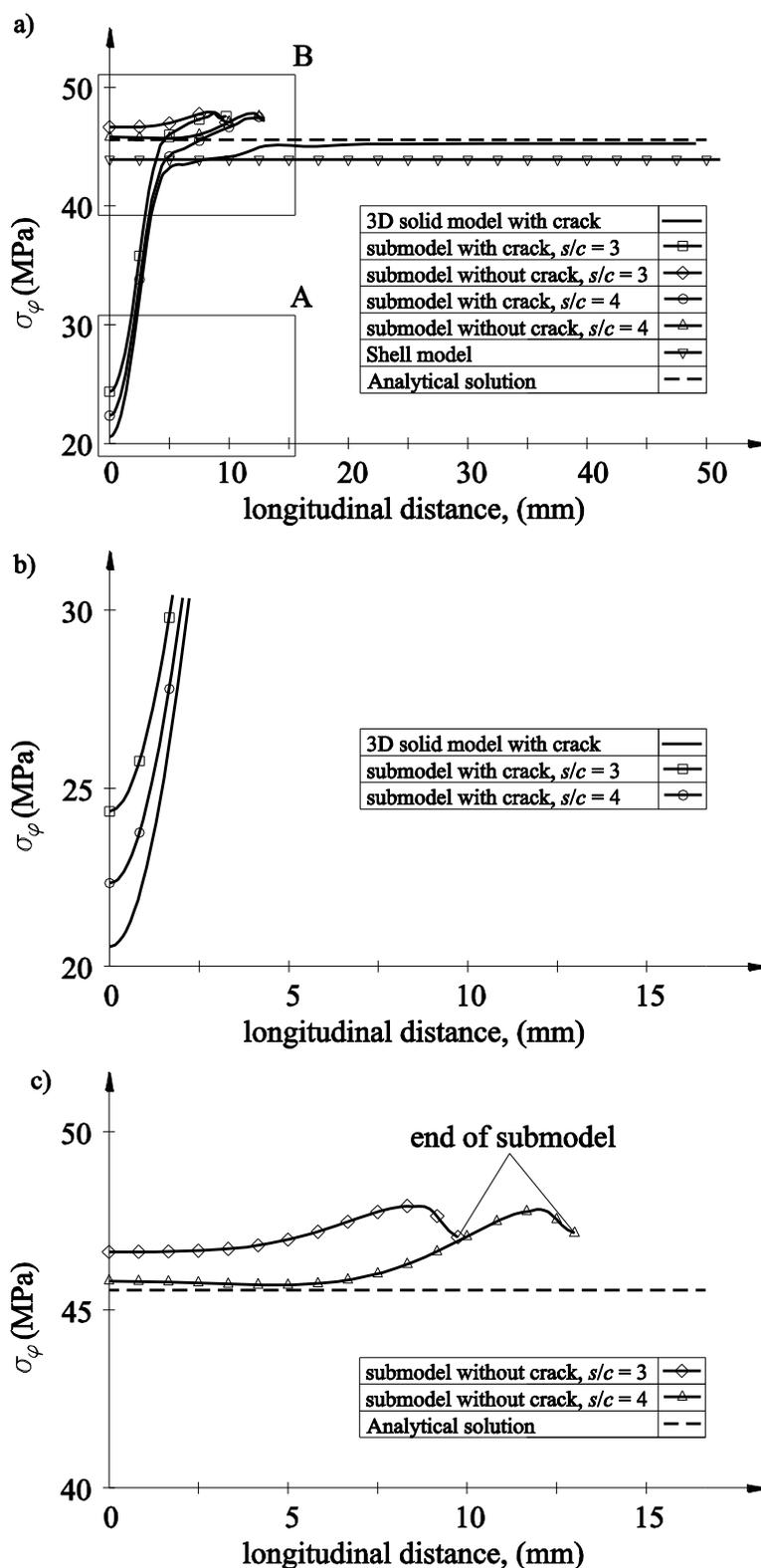
**Fig. 14** a) Hoop stresses distribution of inner surface of the pipe along a longitudinal cross-section ( $R_i/t = 4, c/a = 5, a/t = 0.4, t = 1.625$  mm,  $s/c = 3$  and 4),
