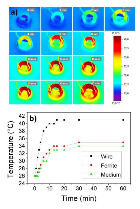
**Figure S3**: (a) Evolution with time of the electromagnet and medium temperature when applying the magnetic field, followed by infrared camera. These experiments were performed in ambient air. (b) Evolution of the temperature in three points of the previous pictures:  $(\blacksquare)$  the wire;  $(\bullet)$  the ferrite near the medium;  $(\triangle)$  the medium.
