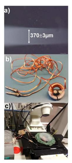
Figure S1: Pictures of the miniaturized electromagnet.
