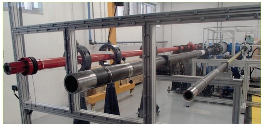
Fig. 14: STIMPACT platform gas guns
