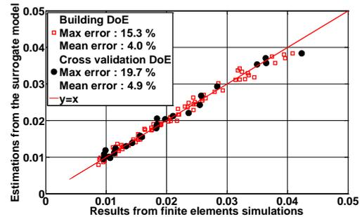
Fig. 7 : Validation of the capacitor thermal model
