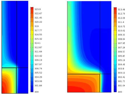
Fig. 5 : Finite elements simulations results for different capacitor geometry (left:  $D/L < 1$ , right:  $D/L > 1$ , temperature scale in °K)
