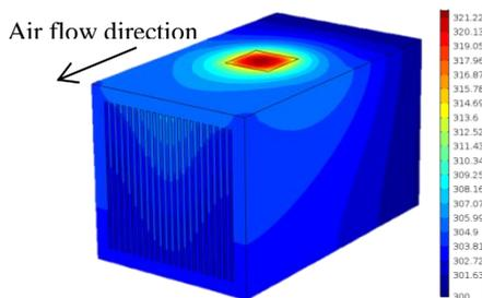
Fig. 8 : Finite elements simulation results for the heatsink model (Temperature scale in °K)
