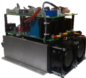
Fig. 3 : DC/AC (one phase) converter prototype
