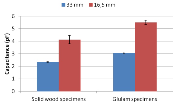
Figure 10: Comparison between results of capacitance measured with different sensor distances (Configuration 4)
