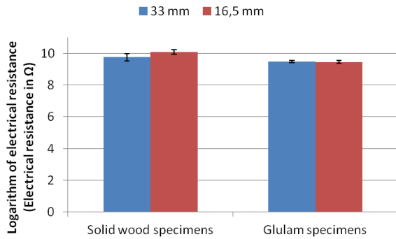
Figure 9: Comparison between results of electrical resistance measured with different sensor distances (Configuration 4)
