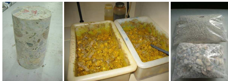
(a) Core samples → (b) Hydrochloric acid attack (1M) → (c) Recovered Aggregate (after sifting)
