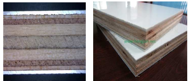
Fig. 3: Allin plywood with aluminium skins.
