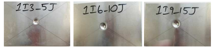
Fig. 6: Plywood with aluminum skins impact pattern.
