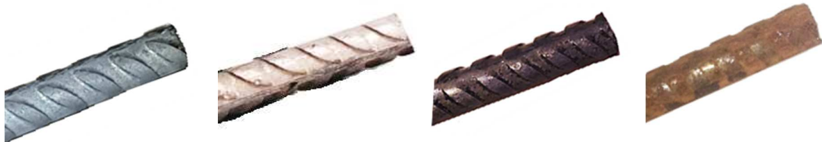
Fig. 2. Different types of steel bars used: ARS, CS, CSPT and CSPH
