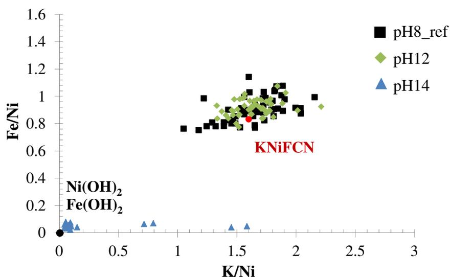
Figure 8: SEM-EDS analysis of KNiFCN product at pH equal 8, 12 and 14.
