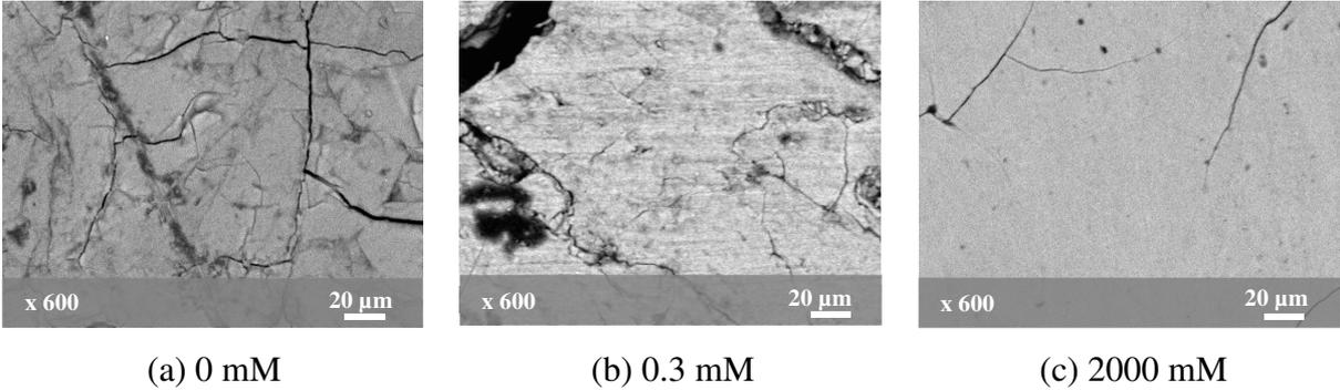
**Figure 1: SEM-BSE images of nickel hexacyanoferrates powder (solid residual) after exposure to different Cs concentrations samples at pH equal 8.**
