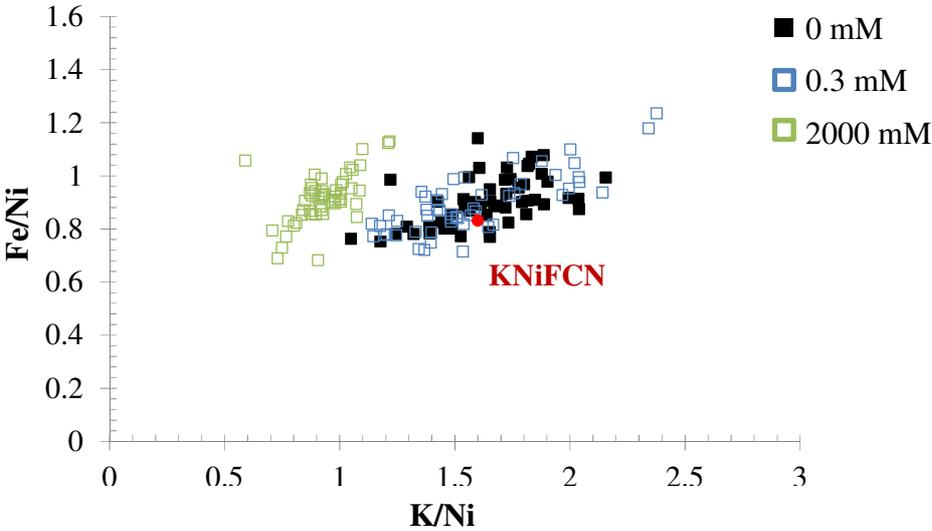
**Figure 2: EDS analysis (50 points) of KNiFCN-Cs samples presented in figure 1 for 0, 0.3 and 2000 mM of Cs.**
