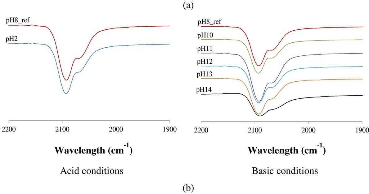
**Figure 13: FTIR spectra of Solution III (2000 mM of Cs) for different pH values of aqueous solution (a) and zooming a section of FTIR spectra around bonding vibrations of KNiFCN products (b).**
