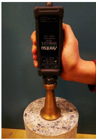
Figure 2. Acquisition of the S_{11} parameter on the surface of a concrete sample.
