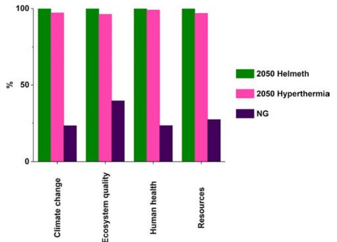
**Fig. 7** Damage categories observed by the LCA of the CO<sub>2</sub> methanation activated by magnetic heating in the 2050 scenario compared with Helmeth project projected in 2050 and natural gas (NG) extraction
