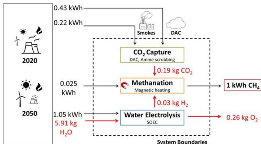
**Table 1** Life cycle inventory of CO<sub>2</sub> capture, water electrolysis and methanation using magnetic hyperthermia in 2020 and projected values toward 2050
