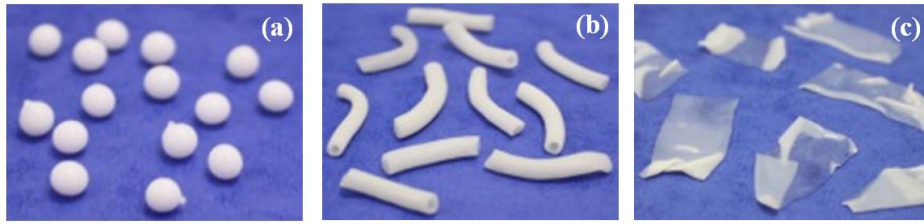
136 137 Figure 2: Photographs of media used in the study: (a) beads (b) hollow cylinders and (c) sheets. 138
