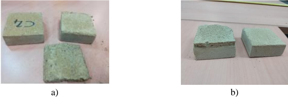
Figure 8: Failure surfaces of Br2 and M2 submitted to direct shear test: a) failure at the interface and detachment of mortar, b) failure at the interface.
