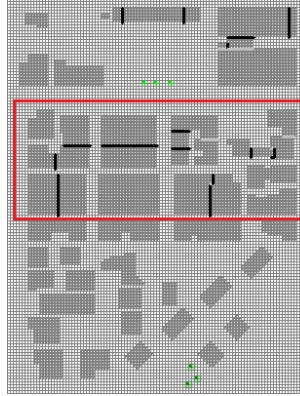
Fig. 5: Sub-model (part of the large model outlined in red) simulated to extract boundary conditions of air temperature and relative humidity.
