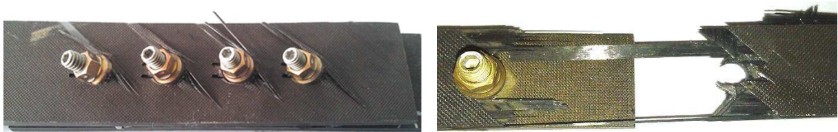
Fig. 11: Failure Patterns of “notched” single lap shear specimens. Left, W = 25 ; right W = 16 (oriented layup).
