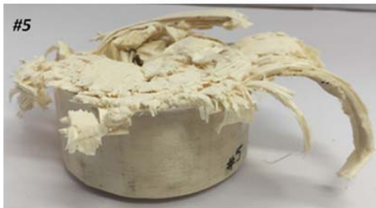
Fig. 15: Petal failure mode for poplar wood.
