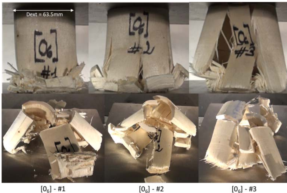
212 Fig. 6: Failure patterns of [0_6] tubes under a crush displacement of 40 mm and post-mortem patterns.
