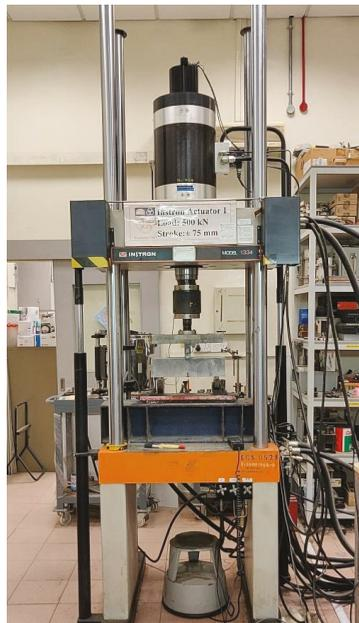
Figure 5. Servo-hydraulic testing machine.
