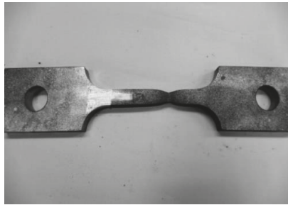
Figure 6. View of tensile failure of S335 steel at ambient temperature.
