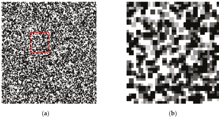
Figure 1. Speckle pattern generated using MATLAB. (a) Complete pattern and (b) magnified view of area highlighted in (a).
