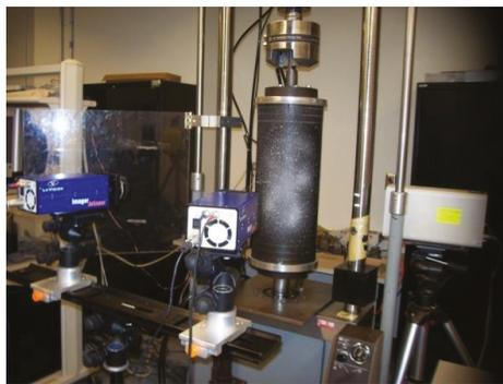
Figure 1. Axial buckling test setup for evaluating DIC [15].
