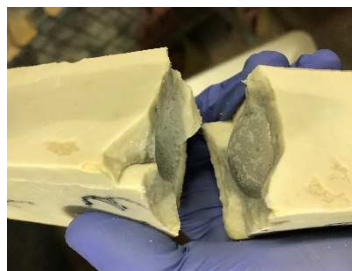
Figure 12: A grout bar of formulation S16-B6.5, broken after passing 90 days in Na 2 SO 4 solution at SO 3 concentration of 3000 mg/L.
