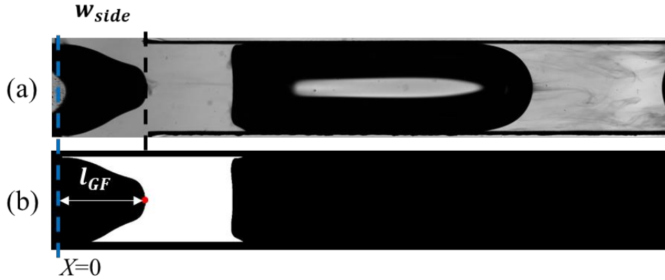
Fig. S 6 Image processing for extracting the length of the gas finger right after the bubble pinch-off ( j_L = 17.9 and j_{G0} = 25.0 \text{ cm s}^{-1} ): (a) raw image of gas finger, (b) extracted gas finger and l_{GF} represents the length of the gas finger.
