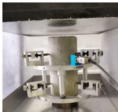
Figure 3. Testing arrangement for modulus of elasticity with cage.
