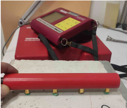
Figure 3: Apparatus for concrete resistivity measurement
