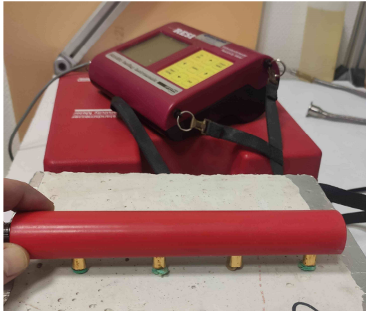
Figure 3: Apparatus for concrete resistivity measurement
