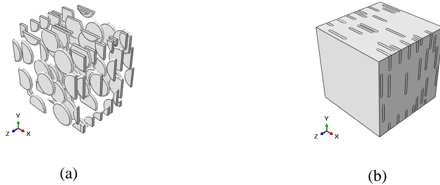
Figure 18 Aligned GPL reinforced RVE for AR=10^{-1} and v_f=0.1 : (a) graphene platelets and (b) numerical model.
