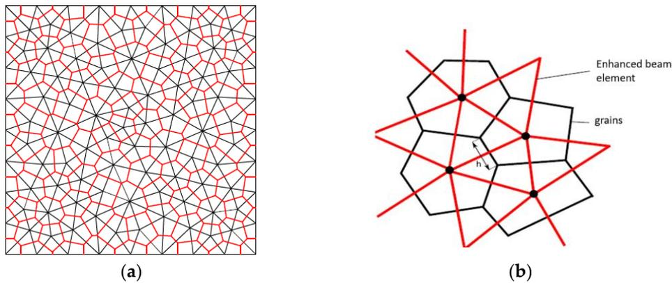
**Figure 1.** (a) Structure of discrete lattice model with Voronoi cells as particles of material and lattice elements. (b) The proposed enhanced beam element connecting neighboring Voronoi cells. Parameter  $h$  is extracted from the Voronoi diagram and represents the height of the beam cross section.
