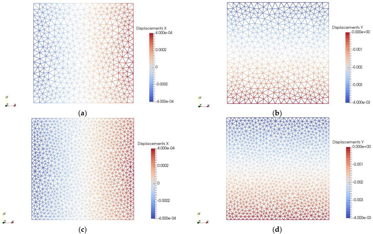
**Figure 15.** Displacement of Voronoi nodes for compression test for imposed displacement 0.004 cm for  $\nu = 0.2$ : (a) displacement in direction x-Mesh1; (b) displacement in direction y-Mesh1; (c) displacement in direction x-Mesh2; (d) displacement in direction y-Mesh2.
