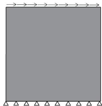
Figure 8. Shear test with boundary conditions.
