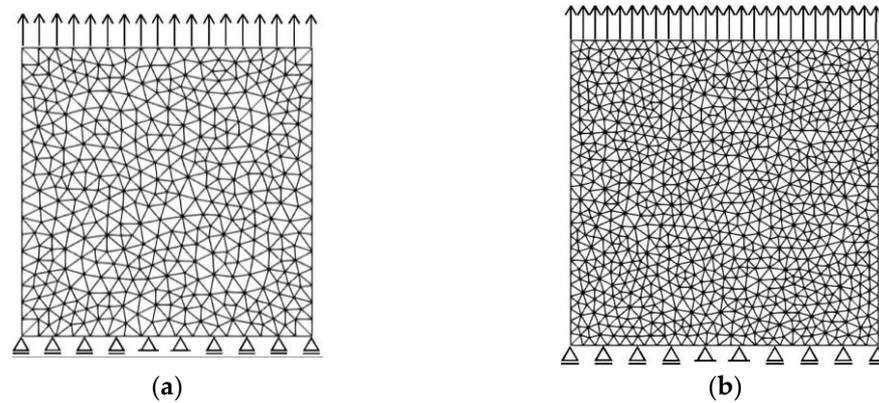
Figure 10. Uniaxial tension test meshes: (a) Mesh1-1210; (b) Mesh2-2570.
