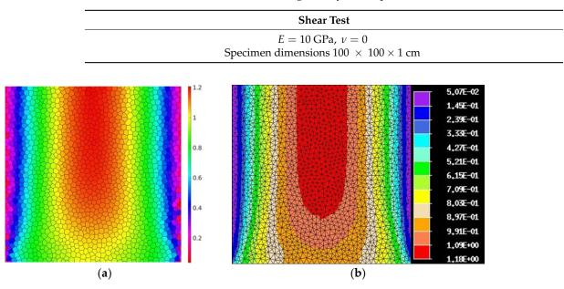
**Figure 9.** Comparison of shear stress state for: (**a**) discrete lattice model; (**b**) FEAP linear solid element (CST).
