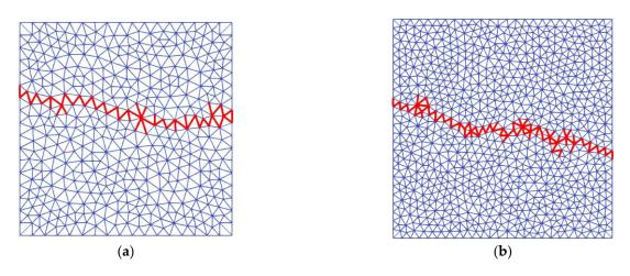
Figure 13. Macro-crack at the end of tension test for: (a) Mesh1-1210; (b) Mesh2-2570.
