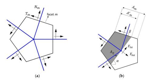
**Figure 4.** (a) Longitudinal and transversal lattice element forces contributing to stress computation; (b) total stress resultant vector acting in the section defined by  $\alpha$ .
