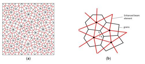
**Figure 1.** (a) Structure of discrete lattice model with Voronoi cells as particles of material and lattice elements. (b) The proposed enhanced beam element connecting neighboring Voronoi cells. Parameter *h* is extracted from the Voronoi diagram and represents the height of the beam cross section.
