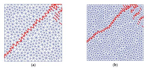
Figure 17. Macro-crack at the end of compression test for: (a) Mesh1-1210; (b) Mesh2-2570.
