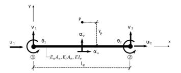
Figure 3. Generalized beam element.
