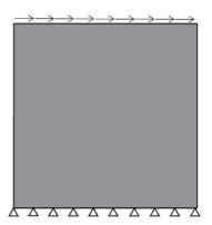
Figure 8. Shear test with boundary conditions.
