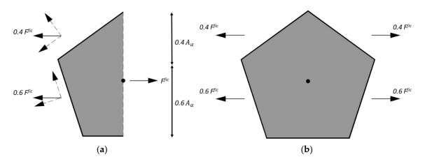
**Figure 6.** (a) The cut plane through the Voronoi cell for computation of nodal fictitious force. (b) The distribution of nodal fictitious forces on a cell.
