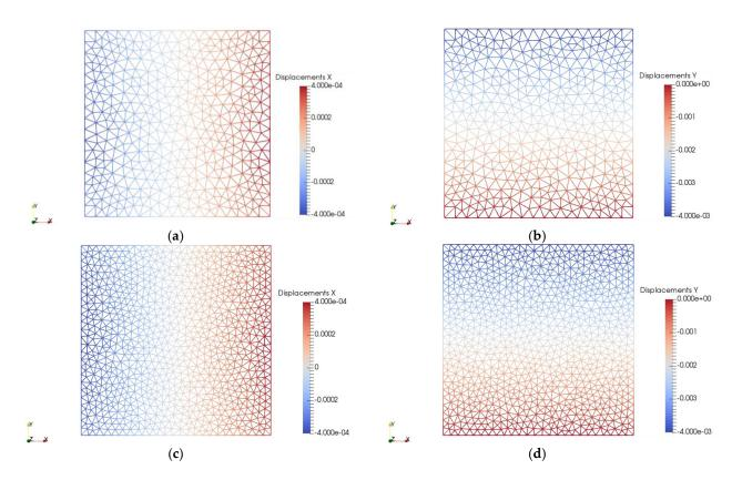
**Figure 15.** Displacement of Voronoi nodes for compression test for imposed displacement 0.004 cm for v = 0.2: (a) displacement in direction x-Mesh1; (b) displacement in direction y-Mesh1; (c) displacement in direction x-Mesh2; (d) displacement in direction y-Mesh2.
