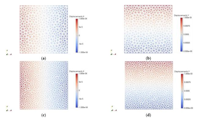
**Figure 12.** Displacement of Voronoi nodes for tension test for imposed displacement 0.001 cm for  $\nu = 0.2$ : (a) displacement in direction x-Mesh1; (b) displacement in direction y-Mesh1; (c) displacement in direction x-Mesh2; (d) displacement in direction y-Mesh2.
