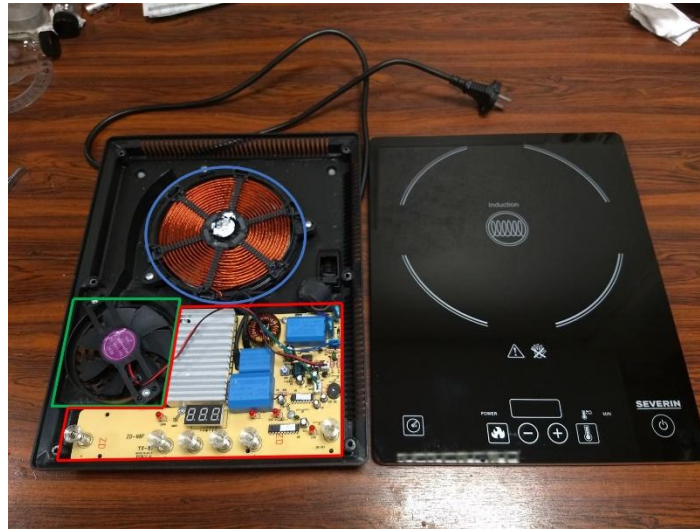
Figure 2: (left) Components inside the housing: electronic board (red), coil (blue), and fan (green). (right) Top part of the housing made of glass-ceramics.
